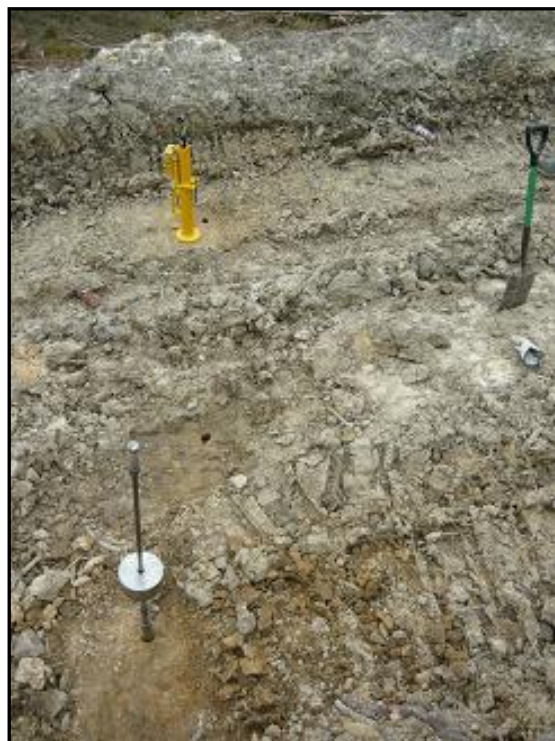
Figure 1. Three sample plots with the Clegg tester (rear) and core cutter (front).
