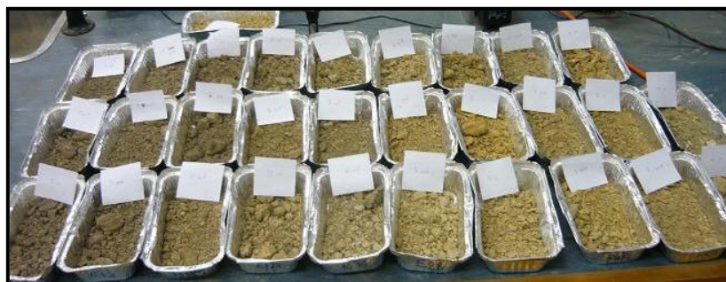
Figure 3. Core samples ordered by colour. Eight samples (left) consist of predominantly organic material.
