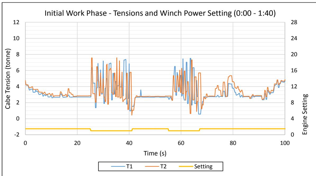
Figure 4: Tensions and winch power setting during initial work phase #1
