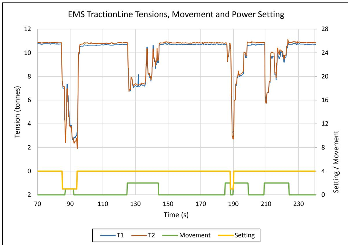
Figure 13: Tension data with power setting and movement data overlays
