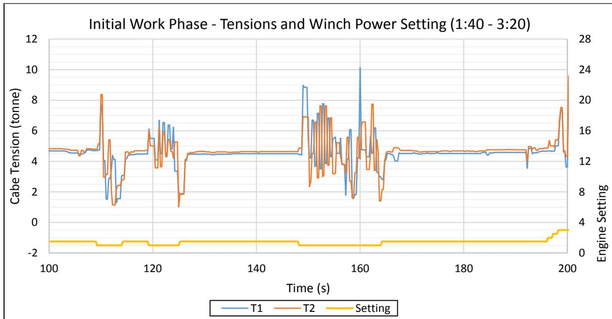
Figure 5: Tensions and winch power setting during initial work phase #2
