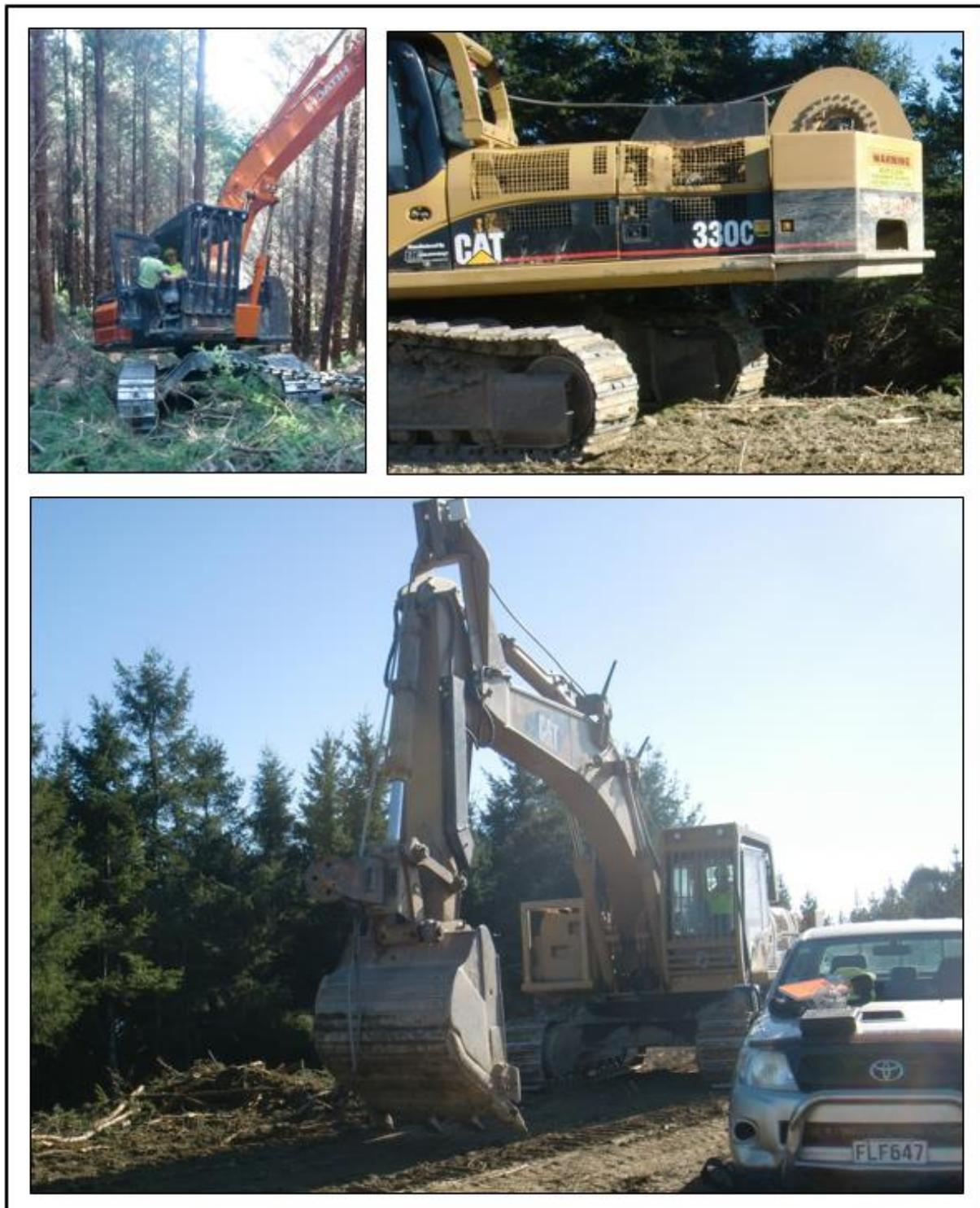
*Figure 3: DC Falcon Winch Assist CAT 330C anchor machine and Hitachi harvester*
