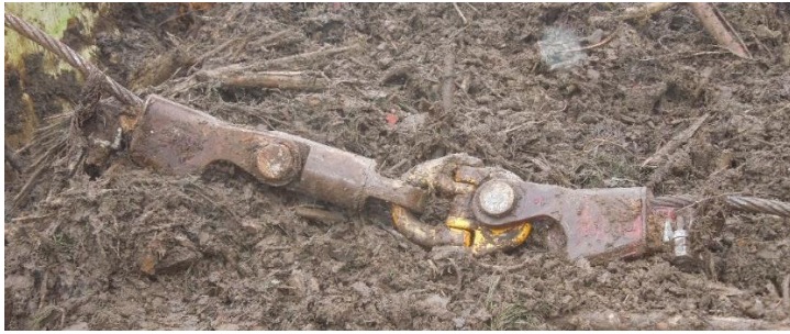
Figure 3: Wedged sockets, hammerlock and swivel system connecting working rope to equaliser section
