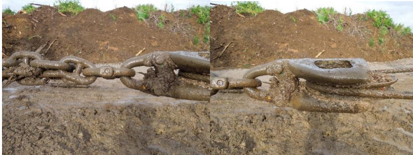
Figure 4: Equaliser block and hammerlock system used for the rope end connection of system 3
