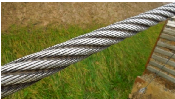
Figure 7: Cleaned section of rope from system 4. Note lack of discernible wear
