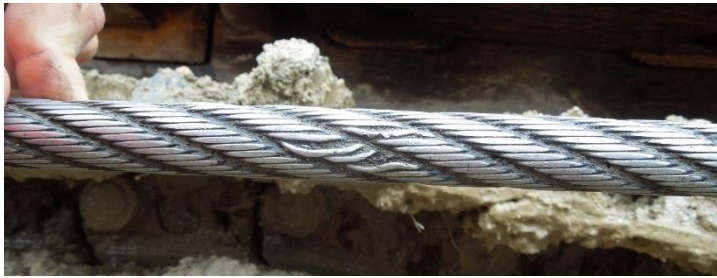
Figure 10: The mechanical damage resulting in failure of the LH rope in system 6
