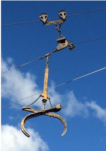
Figure 16: Close up of HeliHawk Grapple logging setup
