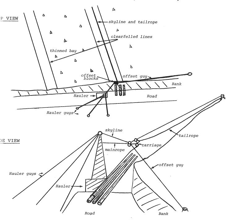
There must be sufficient lift to maintain the skyline well clear of the ground, as this offsetting reduces the effective hauler tower height.
