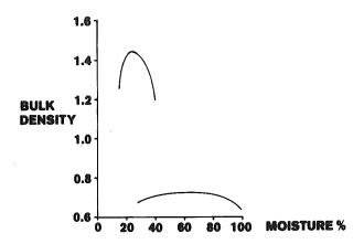
Next, "How do different soils react to logging traffic?". The Soils and Site Amendment Group at FRI have looked at 15 soil types for us so far. These are the sort of charts they are producing for us; they are called Proctor curves. The top curve is for a clay soil in Maramarua State Forest. The bottom curve is for a pumice soil in Kaingaroa State Forest.
