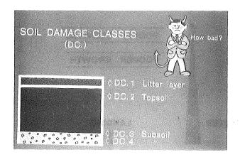
A five class visual system is now used. Disturbance class 0 - the machinery hasen't been over the area. DC1 - machinery has been over the area but didn't break through the litter layer. DC2 - the litter has been broken through and the topsoil is exposed. DC3 - the topsoil has been broken through and the subsoil is exposed. And, DC4 - the machinery has cut deeply into the subsoil.
