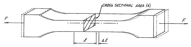
This change in length is referred to as engineering strain and is defined as  $\frac{\text{change in length }(\Delta l)}{\text{change in length }(\Delta l)}$
