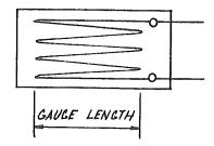
If the gauge is firmly attached to the link, as the link changes length when a load is applied, the gauge must also change its length. This change in length alters the electrical resistance of the "wire" grid. By connecting the gauge to suitable electronics this change in resistance can be converted into an electrical signal.
