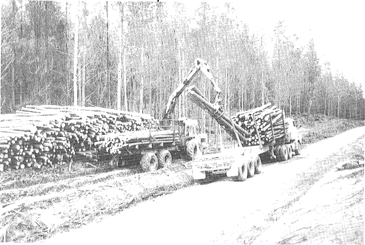
A distinct advantage of the forwarder is its ability to offload itself at the landing, either into wood stacks or directly on to truck and trailer.
