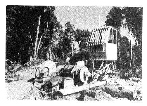
These units can be modernised and improved in a number of ways, at a reasonable cost. This machine has been re-powered, with air controls and a better cab added. Mobility wasn't considered important, so nothing was done.
