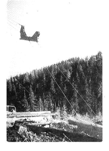
Where you have the advantage of gravity, there are a number of carriages that can be used, from the very simple like this shotgun carriage, to the more complex.
