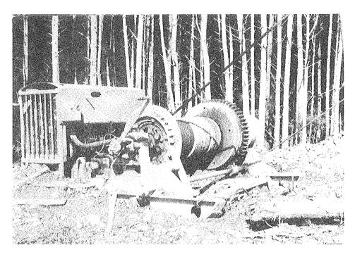
An additional drum for a skyline doesn't have to be mounted on the hauler. A realistic alternative for the older two drum machines can be to have an independent drum with its own power source.
