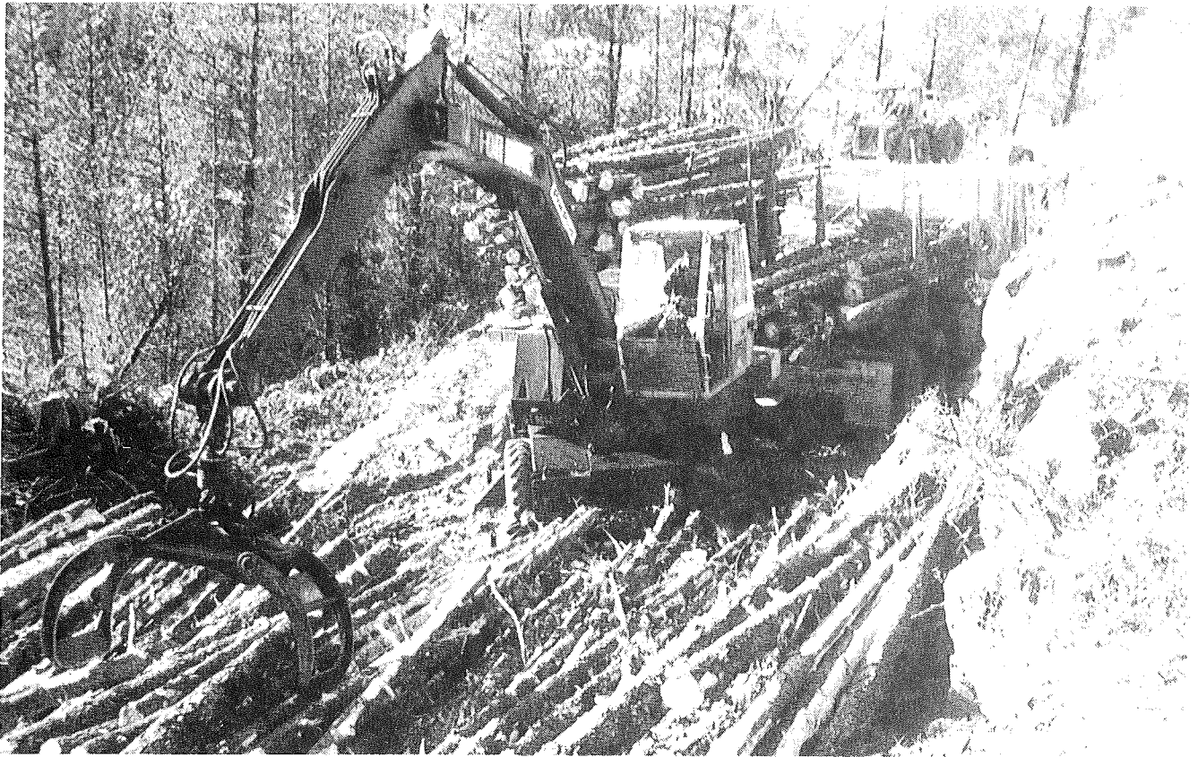
Excavator-based log loaders are well suited to working on landings of restricted size. In this Hanmer Forest operation, the road is the landing.
