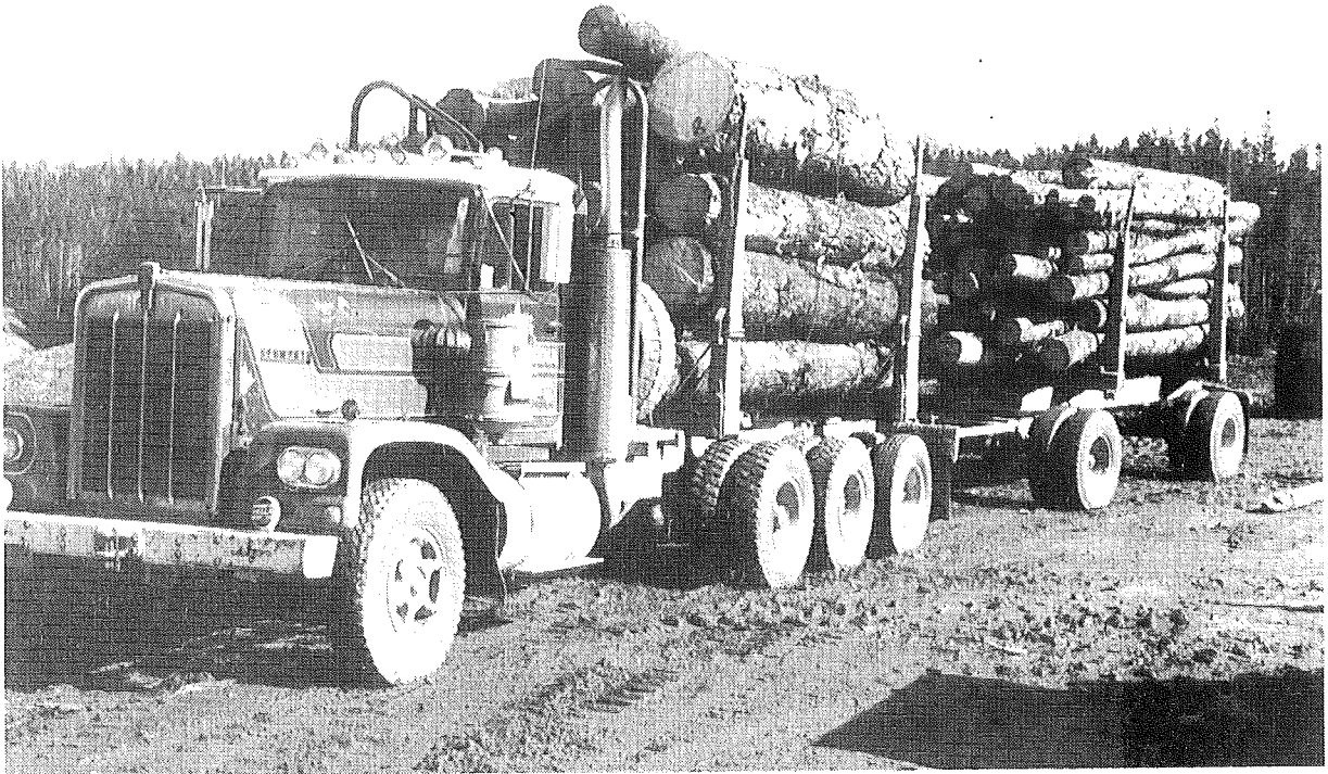
Adding a fourth air suspended axle to a conventional truck (LIRA Photo L345/18)
