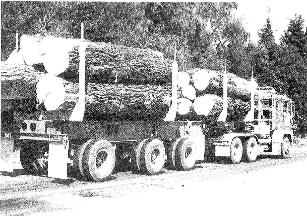
Bailey Bridge type semitrailer units can cart various log lengths (LIRA Photo L325/4)
