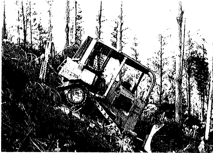
Figure 4 : D4H Tracked Skidder Working on 22° Slopes
