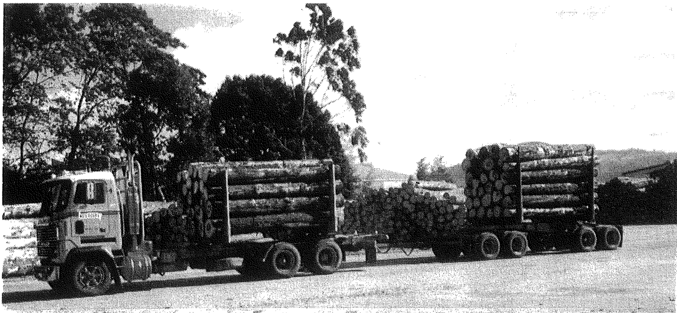
Figure 1 - 6x4 + 4 axle convertible; now able to load to 44 tonnes under the new regulations
