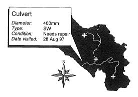
This is one area where GPS has advantages over photogrammetry in that because the features must be visited physically, a lot of useful information can be obtained while the field crew are on the ground. Another feature of this "digital data capture" is that the flow-through of the information eliminates the need for paper notes with later time consuming data entry in the office, and the inevitable errors.
