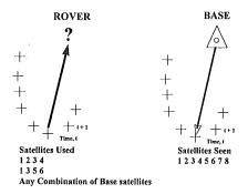
Base station data is available from a variety of sources. In New Zealand there are commercially owned and operated base stations in all of our main centres. For a small fee users can access the base station data externally via a modem or get it posted on a disk. The differential processing is done back in the office using software provided with the GPS.
