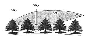
Using planning software supplied with the GPS system, we can make very accurate predictions about the positions of satellites and when there will be a high number overhead. This allows us to plan our activities for a time which will give us the best results. But while this is a good work around, it is not always practical in real life to limit the hours which field crews can work.
