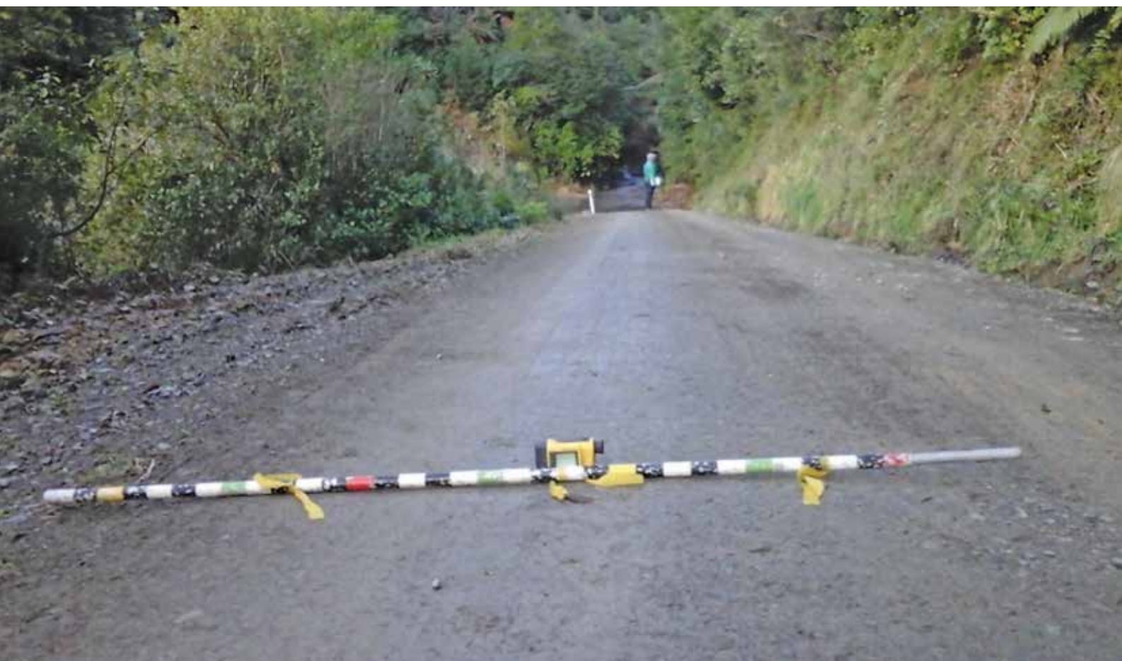
Road camber measurements
