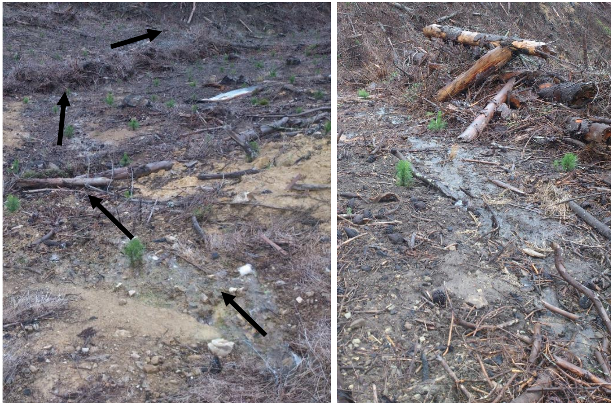
Figure 7. Left: Runoff flowpath on the hillslope below a cross-drain culvert. The slope is moderately steep (21 degrees) and surface cover is low after root raking and replanting, but surface runoff must travel 95 meters on the hillslope and pass through a slash windrow on its way to the stream. Right: Concentrated surface runoff reaches the stream, but it is flowing clean.
