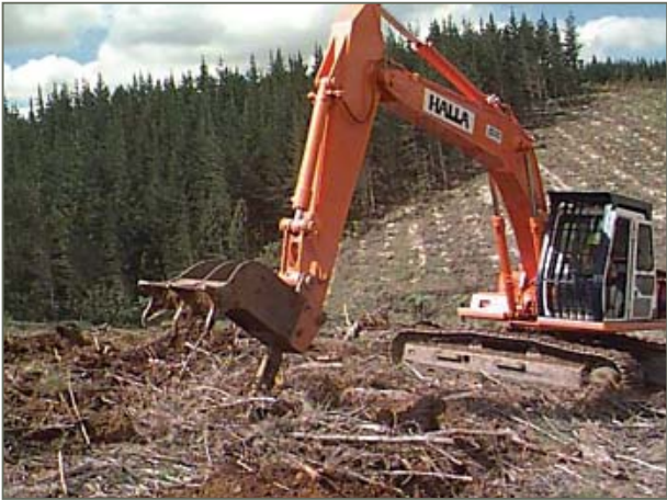
A spot moulder. Spot mounding concentrates the land preparation to the immediate place required.
