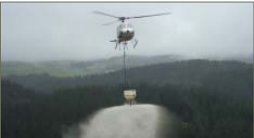
Fertiliser applied by helicopter. A spinner on the bottom of the bucket and GPS navigation for the helicopter enables even, controlled distribution.
