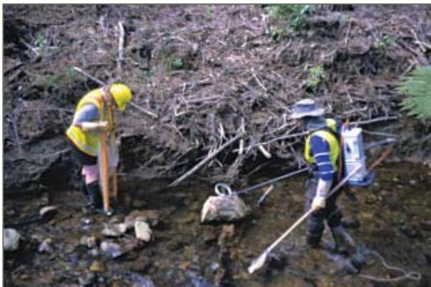
Electric Fishing is a study method useful for identifying the range of fish present in a stream. It can be particularly useful for fish data before and after an activity such as the installation of a culvert.
