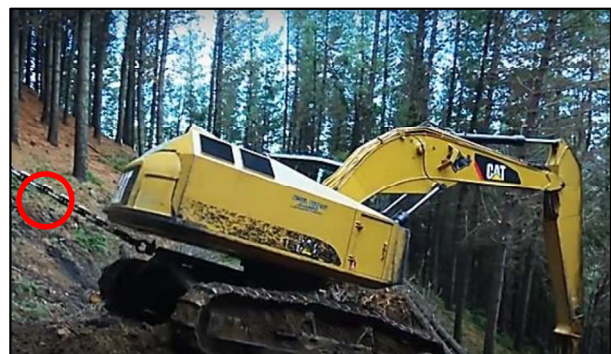
Figure 7. Potential damage point on the connecting chain from the Feller Buncher drawbar https://www.youtube.com/watch?time_continue=124&v=Md8A5E9C9xq (retrieved 27 November 2017)
