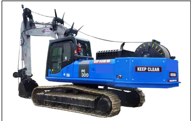
Figure 5. Anchor Machine setup on an excavator https://www.dforestryequipment.com/en/falcon-winch-assist/ (retrieved 27 November 2017)
