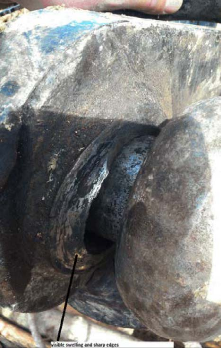
Photo 4: Eye of draw bar, two days before failure, visible signs of swelling and sharp edges
