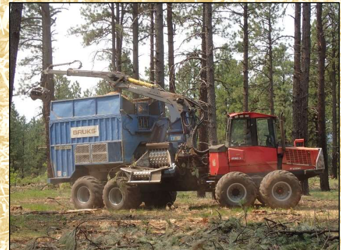
A Bruks chipper operating on a fuel reduction thinning at a study site in southern Colorado
