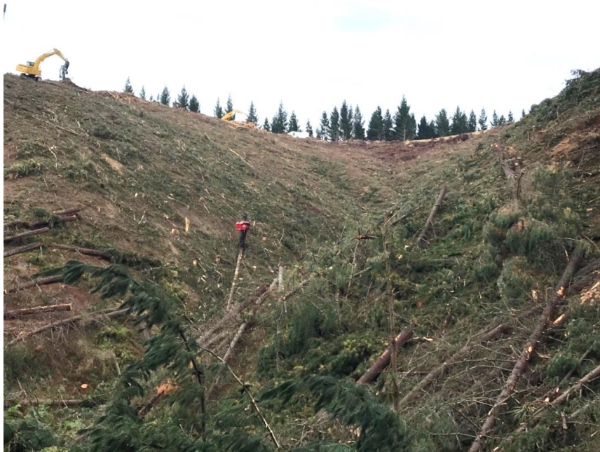
Figure 7: Hawkeye grapple system extracting a stem.
