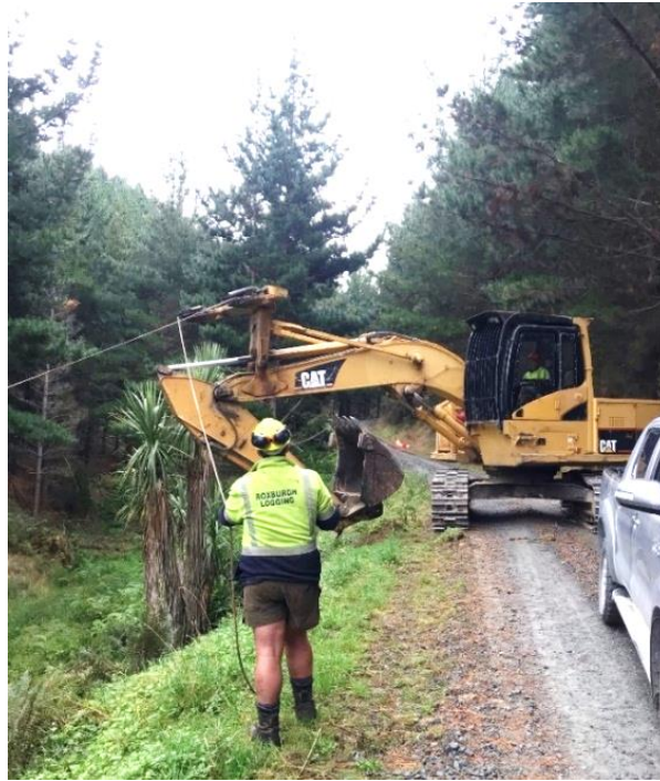
Figure 9: The operator setting up the tailhold machine after a shift.
