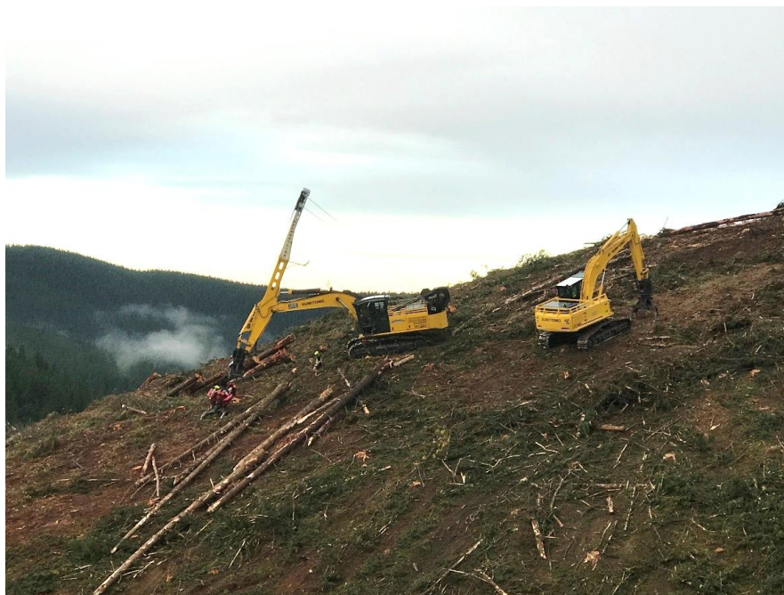
Figure 4: Excavator working with the Harvestline to shift stems up the landing.
