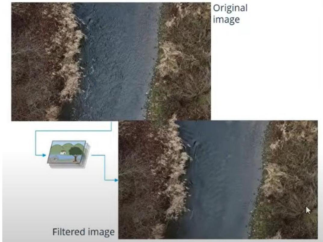
Figure 7. A frame stacking approach to remove surface turbulence
