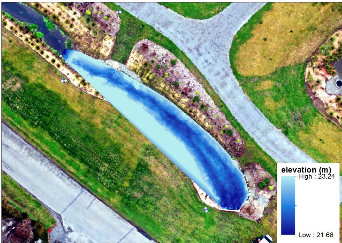
Figure 11. The DEM of the submerged area by small-angle method
