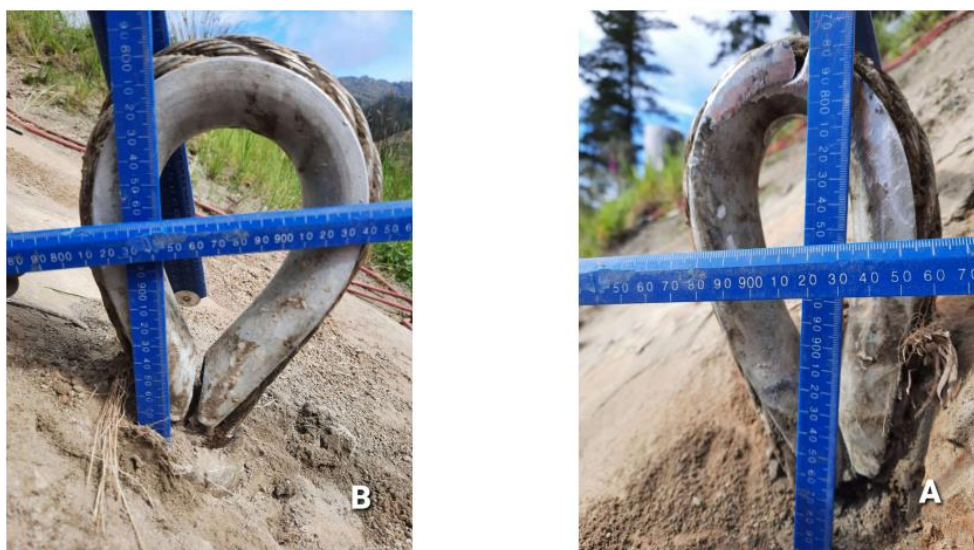
Figure 22 - Thimble displacement occurrence during acceptance testing
