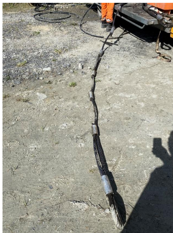
Figure 12 - Wire rope tendon used in testing
