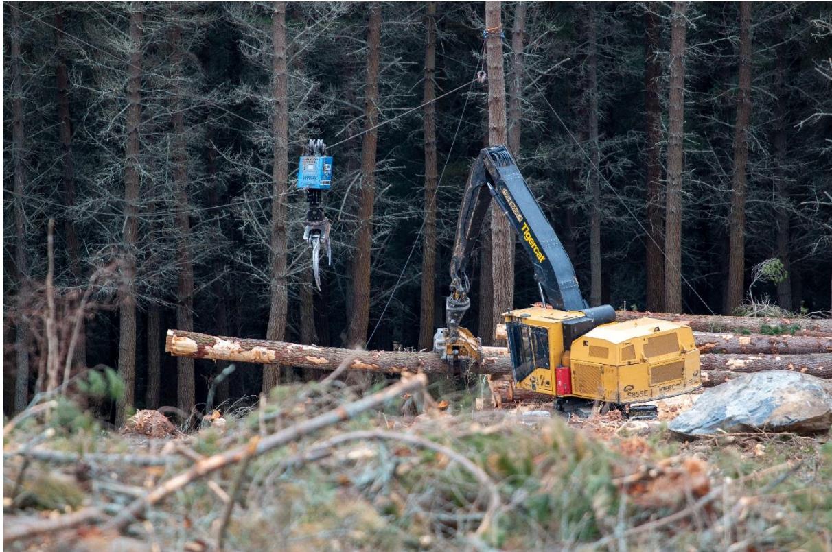
Figure 22: Tigercat LS855E feeding a stem to the Falcon 1750, with tail spar in the background.
