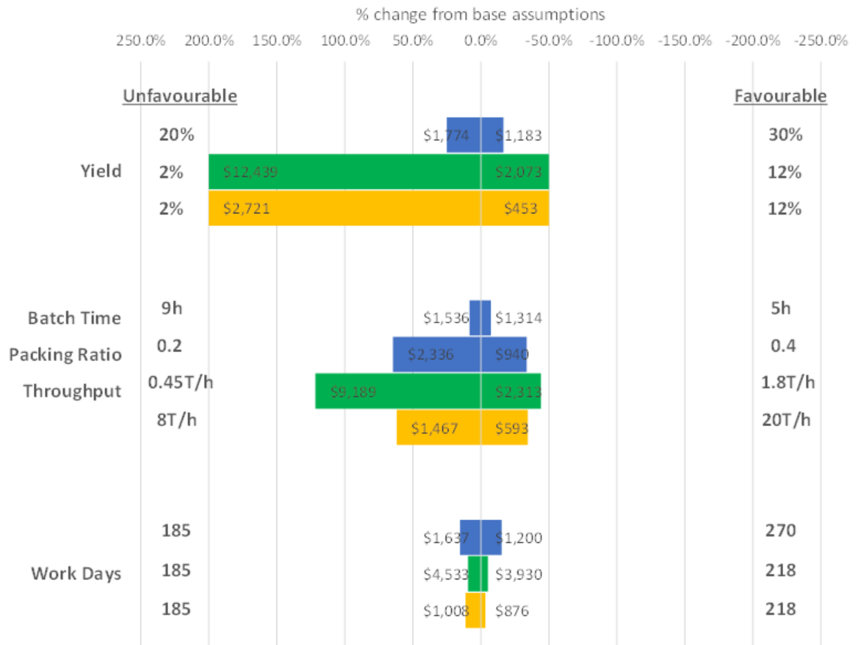
Figure 18. Biochar production cost sensitivity to productivity variables.
