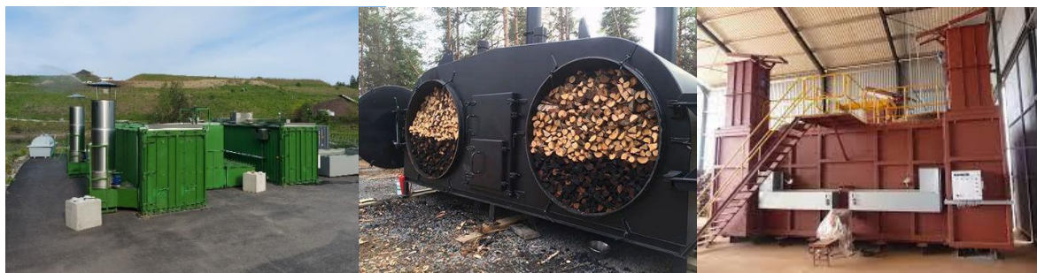
Figure 6. Semi-continuous batch pyrolysis plants (from left) Charmaker FPP by Earth Systems, Custom plant by KTV Enterprises, Twin carbo retort.
