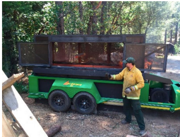
Figure 14. An ember screen fitted to an Air curtain burner to reduce the risk of hot solids escaping (Lee & Han, 2017).
