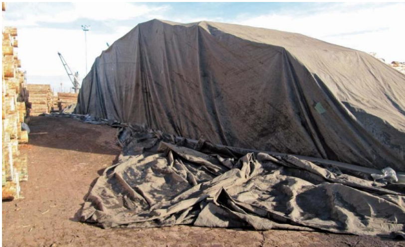
Logs undergoing methyl bromide fumigation under a tarpaulin (Pawson et al., 2014).
