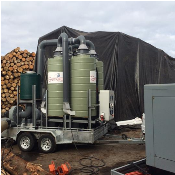
Figure 3: Methyl bromide recapture unit (Genera Biosecurity, 2017).
