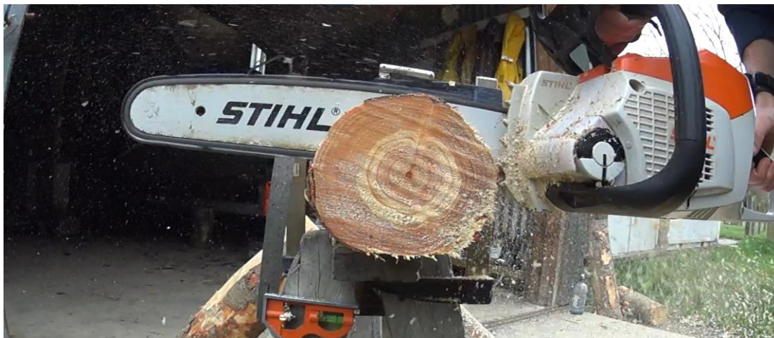
Photo 6: Biscuit being cut during the controlled cutting rate test with the battery-powered Stihl MSA 220c.
