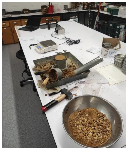
Figure 28: Process of carrying out standard proctor testing.
