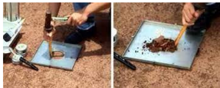
Figure 9: Rubber Balloon Method
