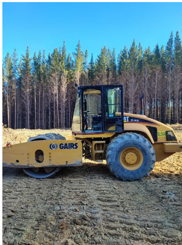
Figure 23: CAT CP-663E padfoot roller used on site 2
