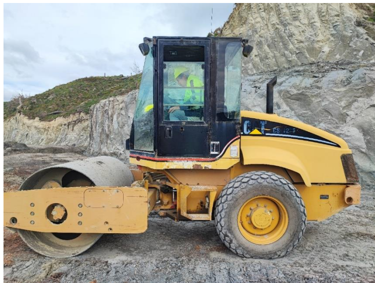
Figure 15: CAT CS-423E which was also used for compaction at site 1.
