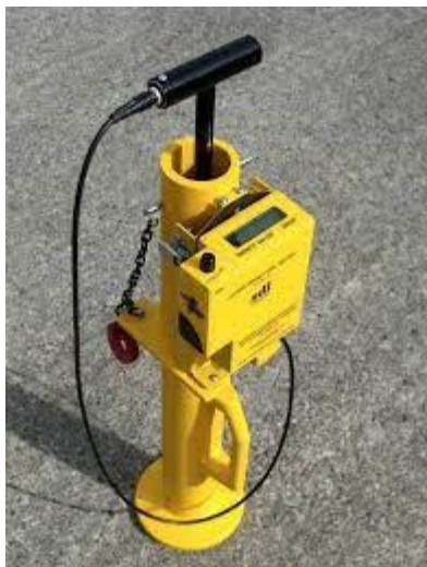
Figure 10: Image of Clegg hammer
