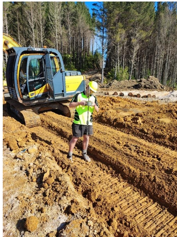
Figure 27: Example image of Scala penetrometer in use following machinery pass.
