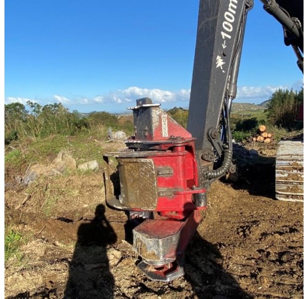
Figure 9 and 10: Lew Prince Logging's felling machine (left). Close up of the felling machines Quadco QB4400 felling head (right).
