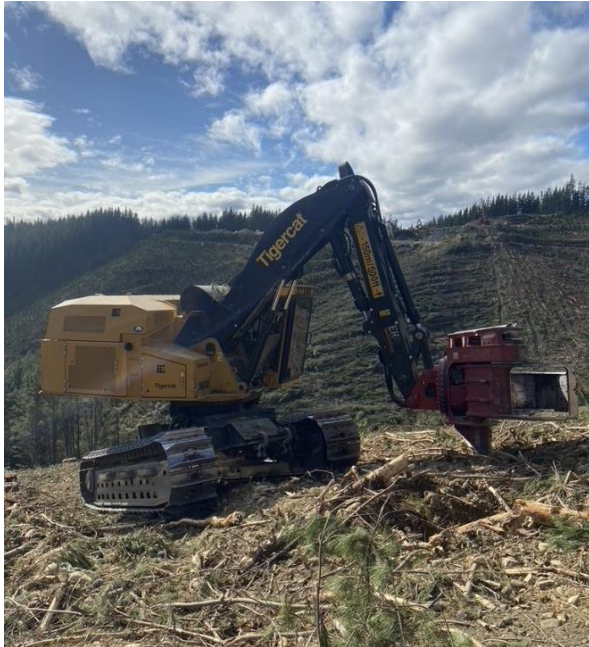
Figure 15 and 16: Endurance Logging/Harmon Harvesting's felling machine (left). Close up photo of the felling machines Quadco 4400QB fixed felling head (right).
