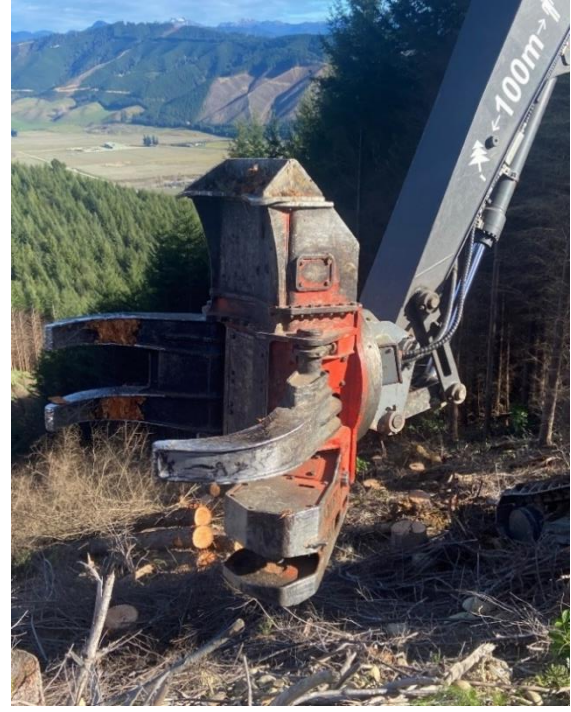
Figure 12 and 13: Hightrack's Felling machine (left). Close up photo of the Woodsman CFH1400 Felling head (right).
