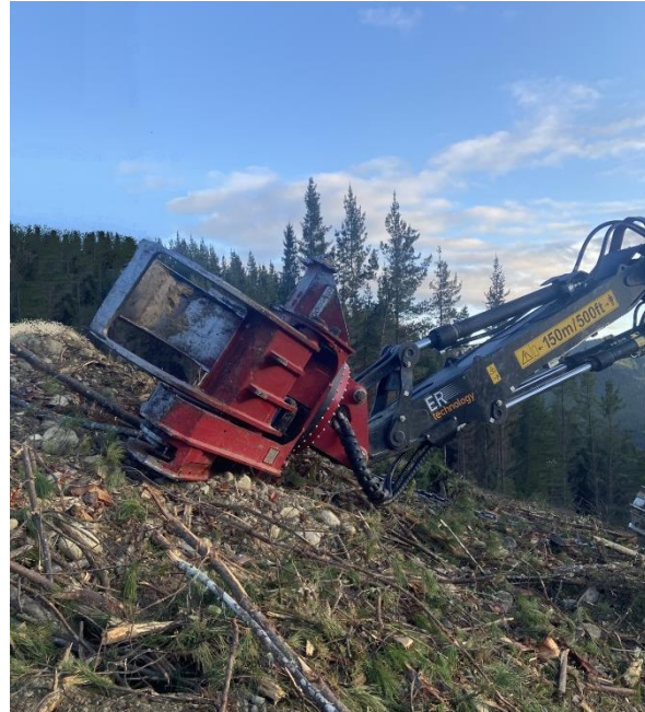
Figure 15 and 16: Endurance Logging/Harmon Harvesting's felling machine (left). Close up photo of the felling machines Quadco 4400QB fixed felling head (right).
