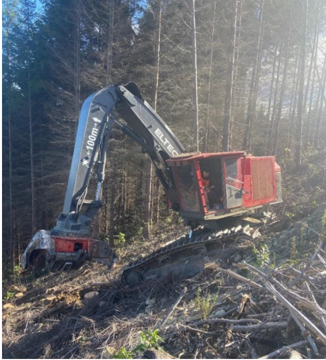
Figure 12 and 13: Hightrack's Felling machine (left). Close up photo of the Woodsman CFH1400 Felling head (right).
