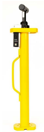
Figure 9: Clegg Hammer testing apparatus (Clegg Hammer, 2022).
