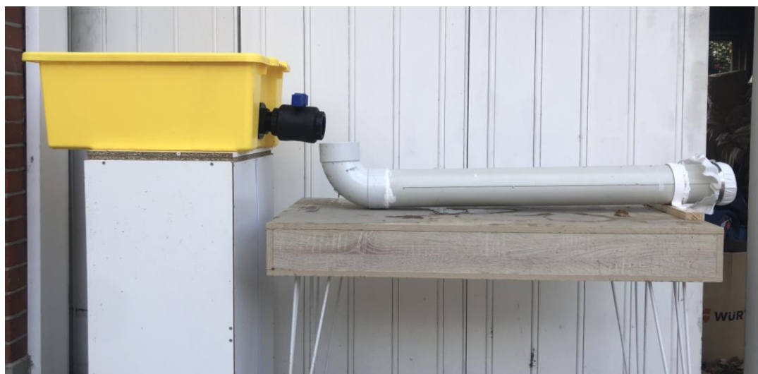
Figure 14: Final working turbulent testing apparatus.
