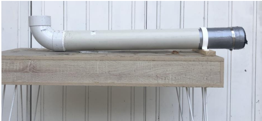
Figure 15: Final working laminar testing apparatus.
