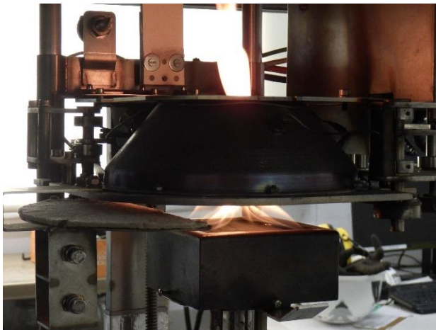
Figure 4 cone calorimetry testing on a sample of E. bosistoana using the method described in the ISO 5660 standard.
