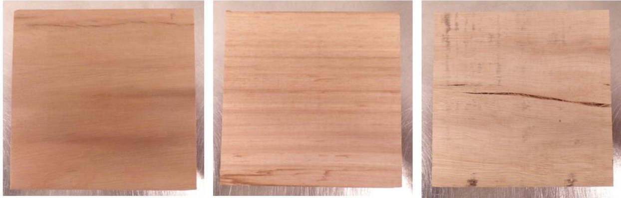
Figure 3 Showcase of samples prepared for cone calorimeter testing: Eucalyptus bosistoana (left), Eucalyptus globoides (center), Eucalyptus nitens (right).
